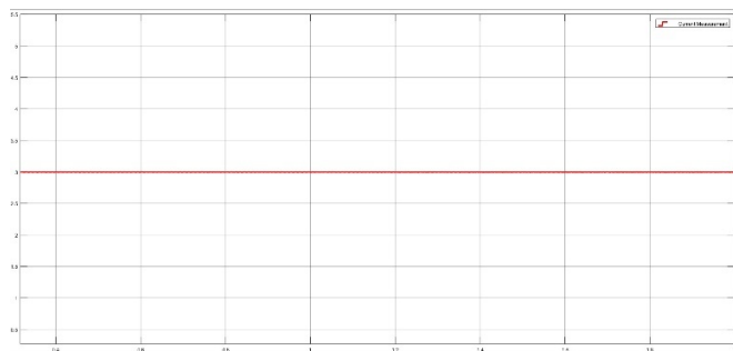
Fig.10. Output current 3A obtained from simulation of Boost converter circuit in MATLAB/Simulink
